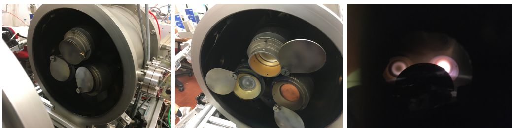
Figure 3.2: Photos of the three torches of the apparatus used for this thesis: with their shutters closed (left) and open (middle). The bottom left torch is a DC one (with an Er target), while the other are RF (the top one has an \text{Al}_2\text{O}_3 target and the bottom right one a \text{SiO}_2 one). The rightmost picture shows the glow of the plasma on the Er torch on the left and the \text{SiO}_2 one on the right during the deposition of an \text{Er}:\text{SiO}_2 layer.
