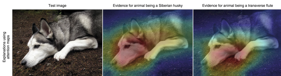
Figure 1.3: Example of saliency map explanation for an image classifier. As the two saliency maps look very similar, there is no way to tell why the network would classify this image as a dog or a musical instrument. Image taken from [Rudin, 2019].
